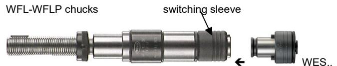
Quick change adaptors with safety clutch type WES.. you always have to combine with tapping chuck with length compensation on compression. Reason: When the safety clutch starts working the length compensation on compression has to take up the rest of the axial movement of the machine to avoid tap breakage while using safety clutch adaptors. The way of compression at the WFL-WFLP chucks usually will be the same as the thread depths or a little bigger then the tapping depth.
