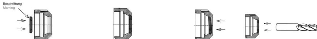
4.5 The tool must be inserted into the chuck at least to the minimum insertion depth. (see table)
