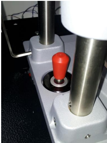
Fig. 6 Inserting the guide unit in the machine
