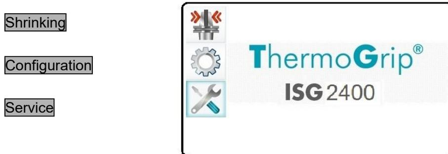
Select with **up ▲** and **▼ down** the function **Service** and activate with **OK**.
