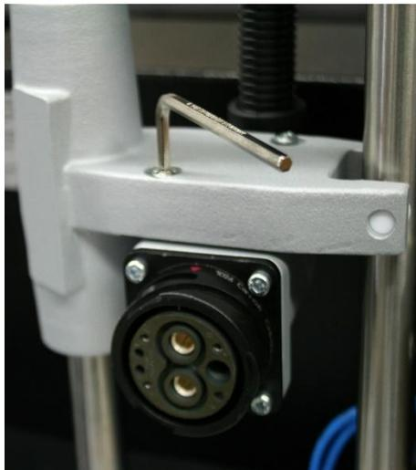
Fasten the connector unit and the cable system to the slide unit with the two enclosed screws (DIN912 M5x20, see Fig. 7).
